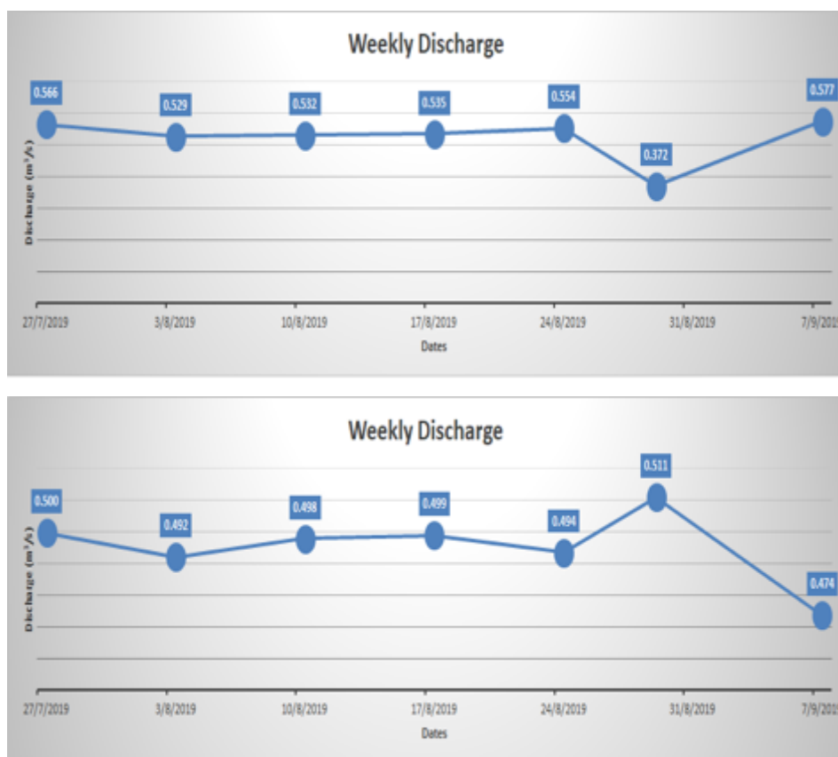
Figure 3. The stream flow during the month of August in 2019 estimated with the use of a current meter in two locations of Ag. Barbara stream (top graph, 1 st location and bottom graph, 2 nd location).
